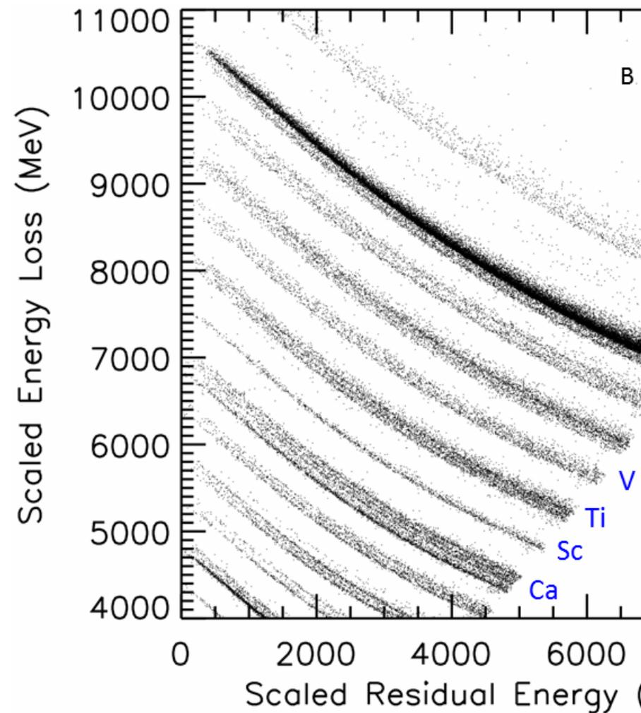
CRIS uses multiple  $dE/dx$  vs. total energy method for charge and mass identification
