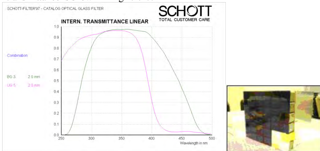
Fig 4.2.17 Transmittance of BG3 baseline filter Green line: BG3 filter
