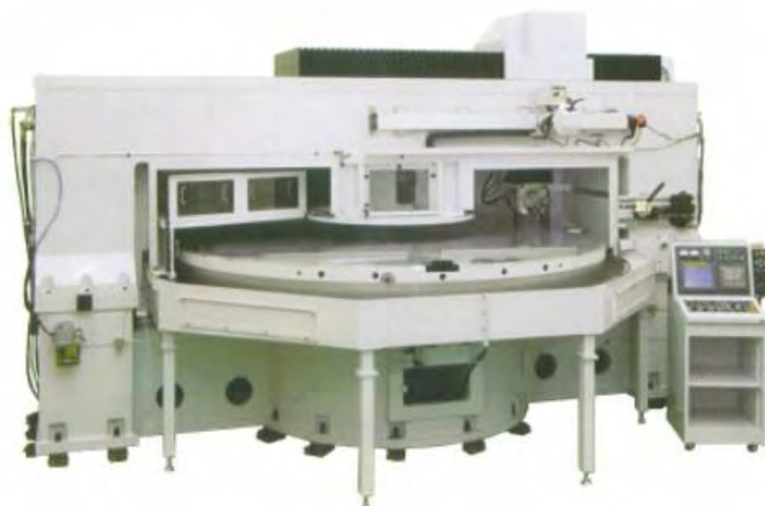
Fig 4.2.21 Large lens manufacturing machine UTD-3400 (Toshiba machine corp.)
