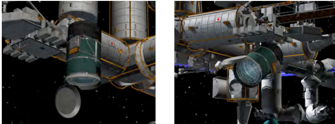
Figure 1-2. Artistic illustration of the JEM-EUSO telescope attached to the Japanese Experiment Module of the International Space Station, under nadir (left) and tilt (right) mode of observation.
