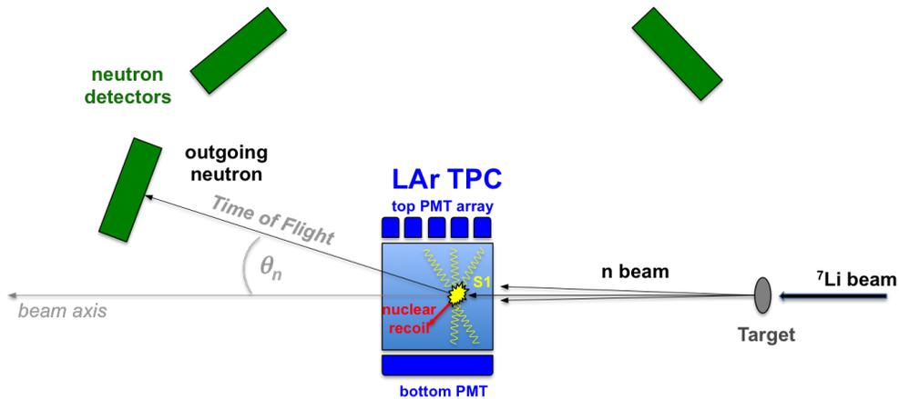
Figure 3: Schematic of the LAr TPC in the neutron beam with neutron detectors (green) at various angles.
