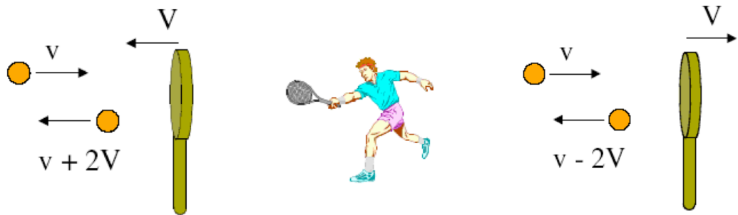
FIG. 3.2: Elastic reflexion of a ball by a wall or a tennis racket. The velocity is conserved during the shock, there is no net change in energy.
